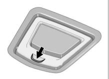
Press the bottom of the load floor handle assembly to lift the top on the handle. Pull up on the handle to open the cargo management system.
